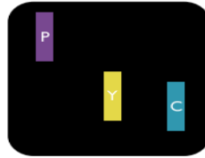
Two adjacent lit sub pixels: red + blue = purple red + green = yellow green + blue = cyan
